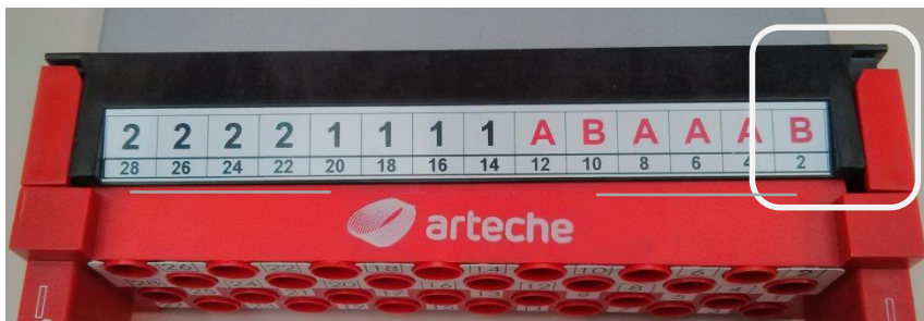
Example test plug incorrectly inserted
