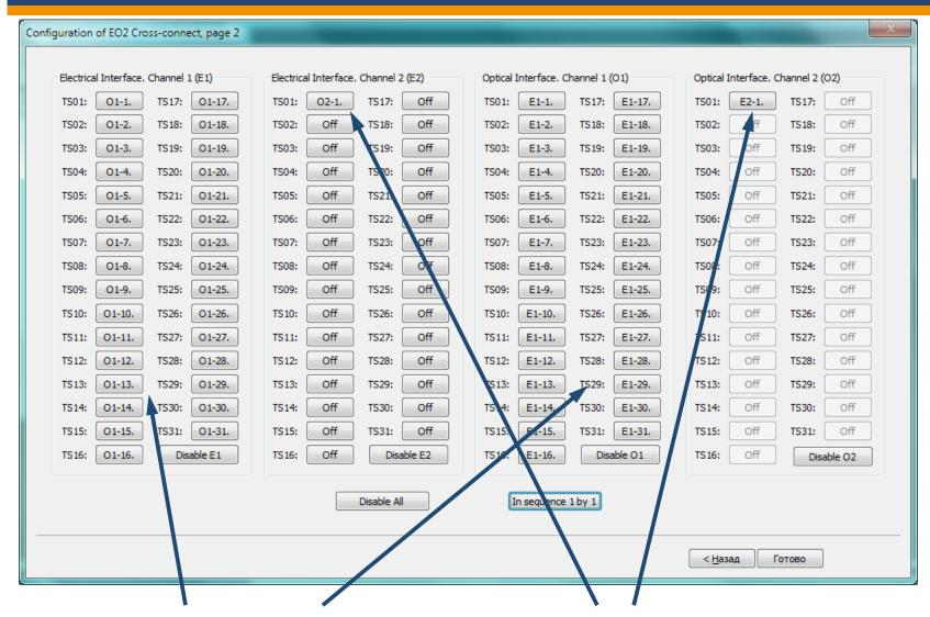
All time slots are transmitted and received between electrical E1 interface 1 and optical interface 1
