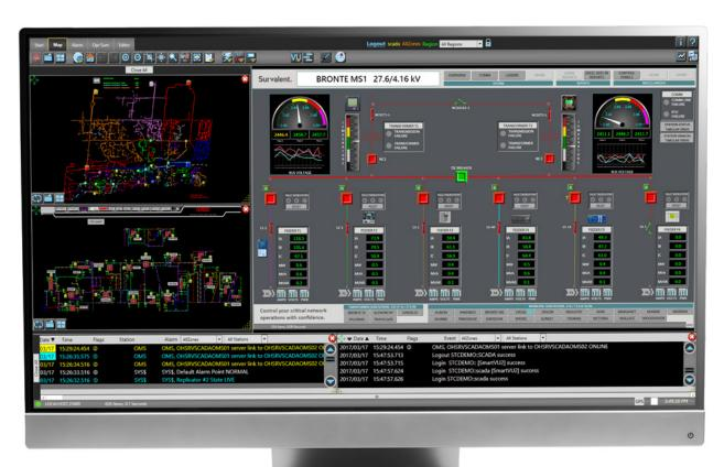
SurvalentONE SCADA can be configured to provide operators with relevant information at a glance. Maps, single line diagrams, schematics, event summaries & alarms are shown in this view.
