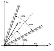
difference between the vectors is within the preset range. The decision enables the output start and trip signal of an overcurrent protection function block (51N/51Ns). This nondirectional residual overcurrent protection function block is described in a separate document. The directional decision module calculates the phase angle between the residual voltage and the residual current. The reference signal is the residual voltage according to the Figure.
