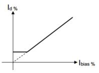
The horizontal axis of the operating characteristic is drawn as the percent of the phase current transformer rated current, the scaling of the vertical axis is in percent of the crated value of the current transformer into the differential branch. As the turn's ratio of the current transformer in the differential branch is much less than that of phase current transformers (one tenth or one over twenty), the decision can be performed in high precision.
