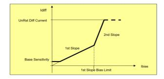
The characteristic curve has four sections. The first section is the base sensitivity, the second one serves to compensate the turns ratio deviation e.g. due to the operation of the on-load tap changer, the third is to eliminate false operation caused by the CT saturation and the fourth one is the unrestricted differential function.
