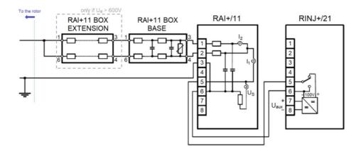
Wiring for ConnType2 (single point connection) mode
