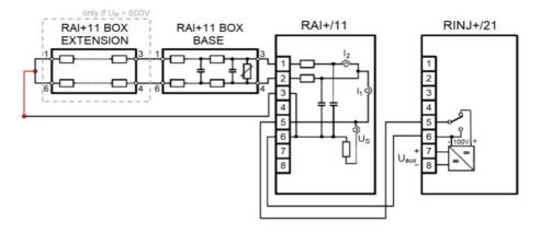
Wiring for Calibration mode
