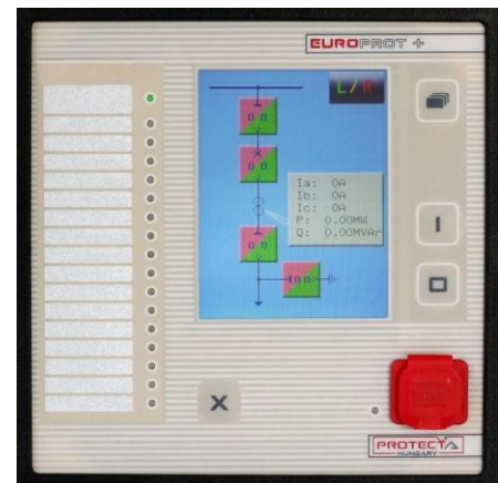
IED EP+S24 True color HMI front panel
